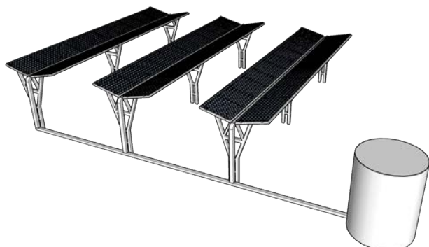
Fig. 49: Concept design for a rainwater harvesting system with storage tank. © Fraunhofer ISE
